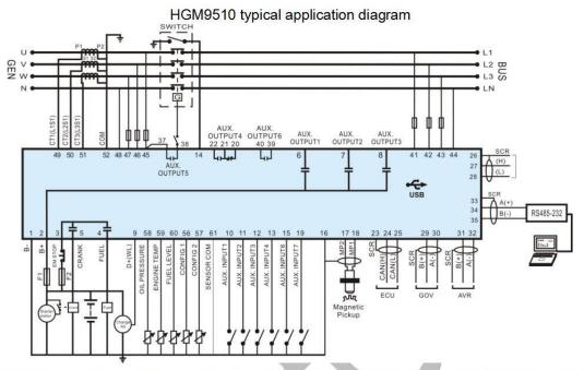
**A**Note: Fuse F1: min. 2A; max. 20A. Fuse F2: max. 32A. Users should select suitable fuse depend on practical application.
